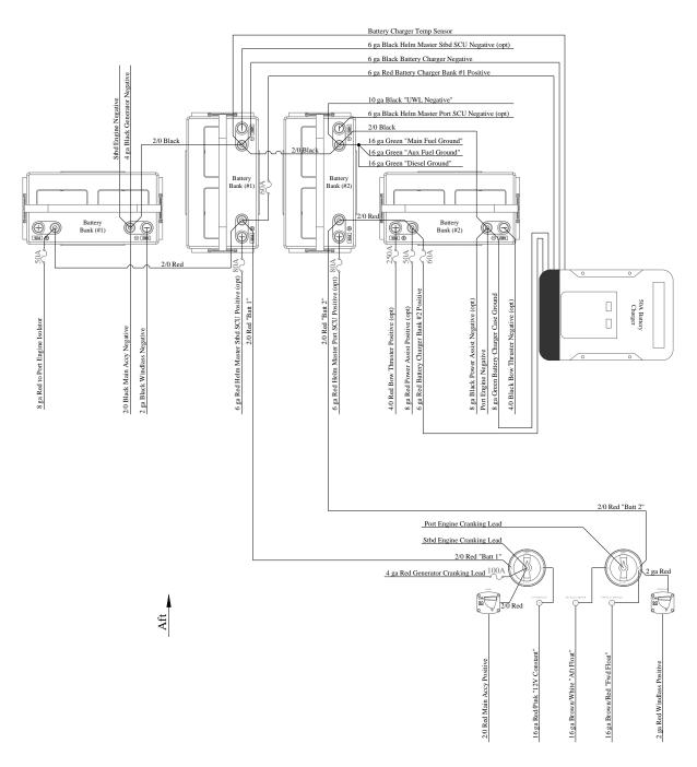
NOTE 1: Engine isolator fuse changes to 100A MRCB if the boat is powered with V6 engines.
